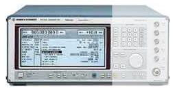
The Rohde & Schwarz, Inc. SME02 signal denerator is an electronic instrument that generates repeating electronic signals. It contains an electronic oscillator, a circuit that is expable of creating a repetitive waveform.
