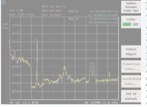
AF spectrum of an FM stereo signal: The 19 kHz pilot carrier, the stereo signal on the 38 kHz subcarrier and the RDS subcarrier at 57 kHz are clearly distinguishable. The pilot deviation is selected using the marker.
