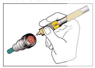
An optional beam collimator (P/N 1601) simplifies fault detection for single- and multi-pin receptacles. The user need only aim the collimated beam into the receptacle to trace faults. This beam collimator is especially useful for tracing faults in multi-channel cables, eliminating the need for a specialized adapter, or disassembly of the connector.
