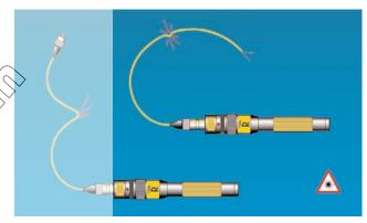
The 160L visual fault finder is an indispensable tool for quickly identifying bending losses and breaks in optical fibers. If a fiber is bent too tightly, red laser light will be seen escaping through the jacket, as shown above, at left. Likewise, if a fiber is broken, escaping light will be visible where the break is located, as shown at right.
