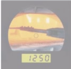
Viewfinder image clearly indicating the measured temperature
