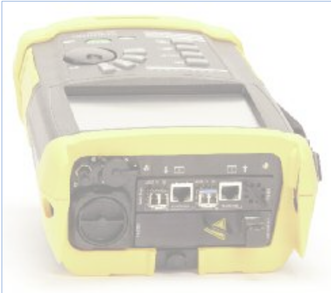
Gigabit Ethernet Module in OV-1000 | Photo TEQ34
