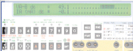
Dual multimeter display showing battery and loop current measurements.
