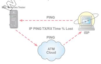
The DSL Services Tester verifies IP layer routing.
